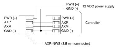
FIG. 6 AXlink and 12 VDC power supply wiring diagram
